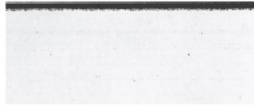
HASTELLOY® B alloy Average Metal Affected = 2.6 Mils (66 \mu\text{m} )
