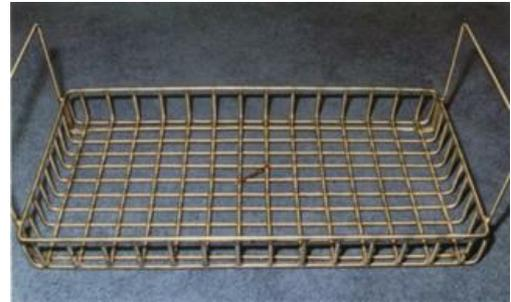
Fabricated heat-treating basket for vacuum furnace application to 2300°F (1260°C). Made from 1/2-inch (12.7 mm) diameter 230<sup>®</sup> bar.
