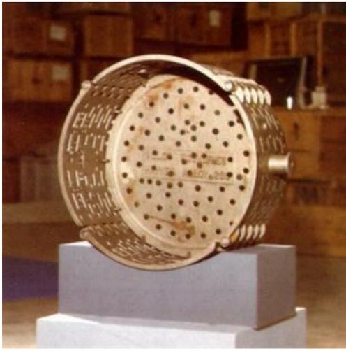
Cast heat-treat basket of 230<sup>®</sup> alloy in use at Alloy Foundries, Division of the Eastern Company, Naugatuck, Connecticut.
