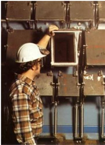
230<sup>®</sup> retorts operate at 2100°F (1150°C) with a hydrogen atmosphere (inside) and combustion products outside.
