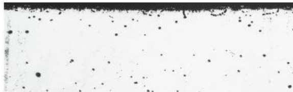
Alloy 600 Average Metal Affected = 4.8 mils (122 \mu m)
